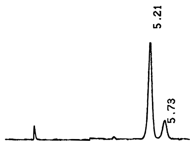
Figure 2. HPLC of 7 in 5% EtOAc in hexane on Nucleosil 50-5.
